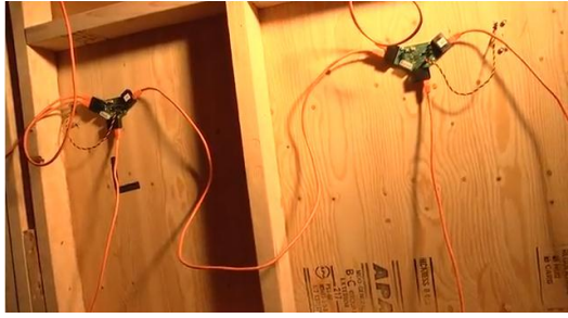
Figure 2. Inside of the “Swarm Wall” showing the wooden structure, PCBs and Ethernet cables.
