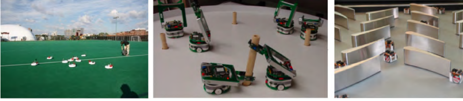
Figure 3.8. Instances of networked robots with hybrid reactive-deliberative controllers. Autonomous deployment of wireless infrastructure ([Correll et al. (2009b)], left), distributed manipulation ([Martinoli et al. (2004)], middle), and inspection of regular structures ([Correll and Martinoli (2006a)], right). The spatio-temporal behavior of each of these systems is generated from the interplay of reactive controllers and discrete state transitions at the individual controller level.
