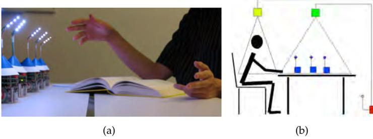
**Figure 8.2.** (a) A networked multi-robot system forms a reconfigurable interactive table lamp, assuming various configurations based on user activity or input. (b) Interaction setup. Robot and user positions are tracked using two different tracking systems. The information is then combined and sent via radio packets to the robots, which take action accordingly.
